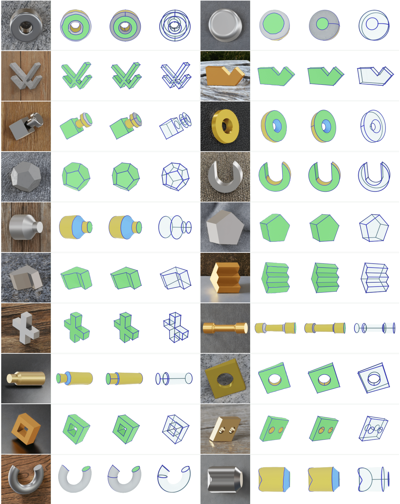
Figure 10. Reconstruction results from the given images are shown from left to right: input image, reconstructed mesh, B-reps, and their CAD vertices and edges. Different colors indicate different primitives: plane (●), cylinder (●), cone (●), sphere (●), and torus (●).
